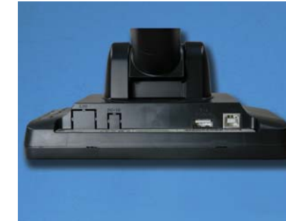
Two USB ports are located under the display panel to facilitate simple image updates.
