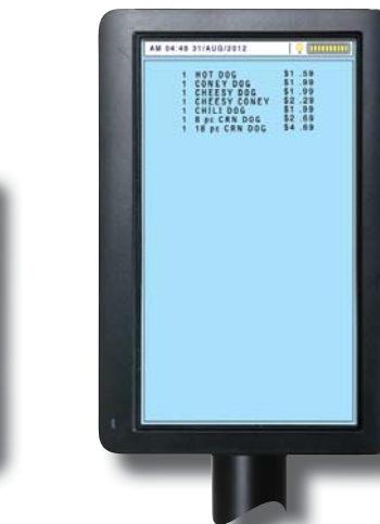
Rotate the screen for three portrait configurations. The SAM4s ML700 automatically senses portrait mode.
