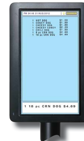
Rotate the screen for three portrait configurations. The SAM4s ML700 automatically senses portrait mode.
