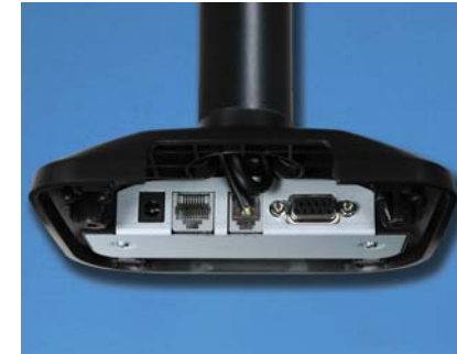
Easily accessible ports are located in the base.
